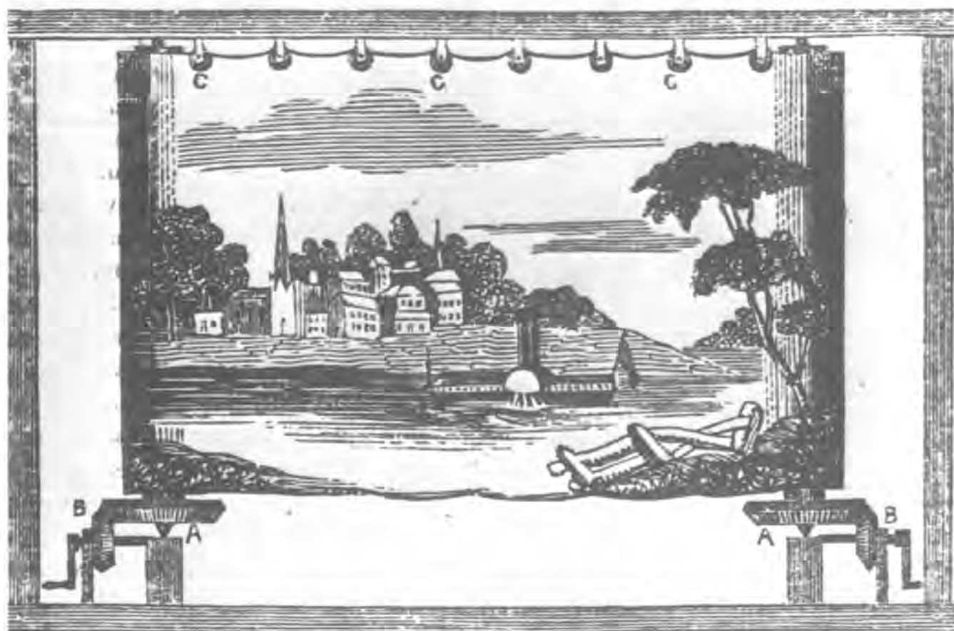
Fig. 2. Woodcut illustrating the machinery for Banvard's moving panorama, Scientific American (December 16, 1848).
